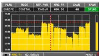
Spectrum TV 100 MHz span
