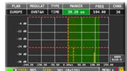
ECHO MEASUREMENT in SFN networks, with impulse response in real time, green area shows the guard interval
